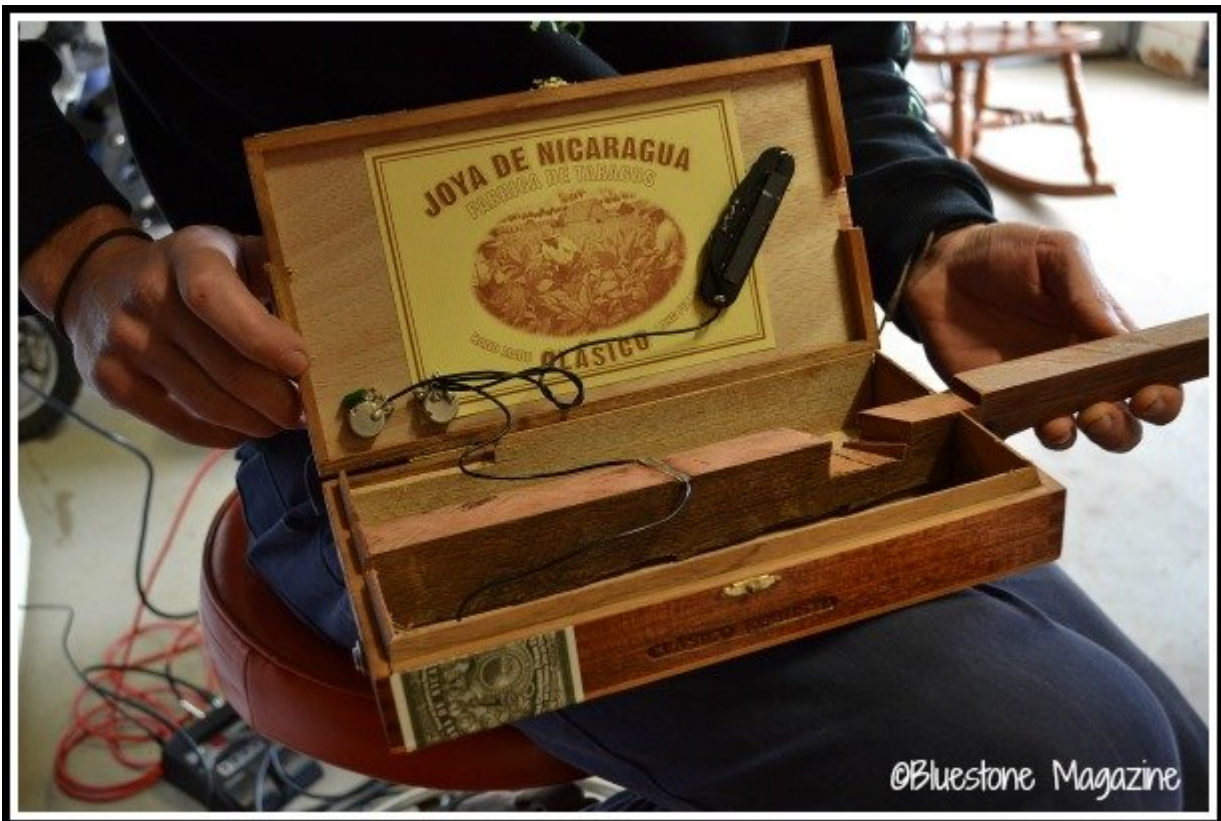
Simple but effective. This cigar box guitar made by Brendan includes volume and tone controls and can be used with an amp.
