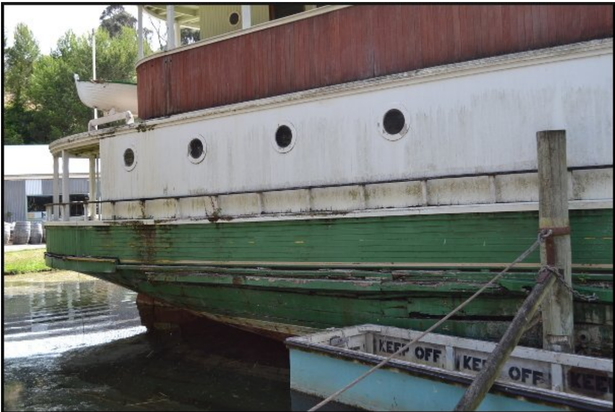
The rotting hull of the Rowitta, which has been off-limits to visitors to Flagstaff Hill Maritime Village for more than a year.
